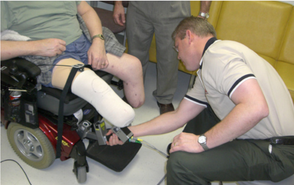
The BioScanner™ from the BioSculptor System™ operates with dual cameras and a laser imager, mapping precise measurements. This technology is available to all NOPS patients.
